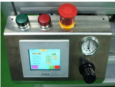
Color Touch Screen HMI is installed; operation is easier. All setting and parameters are input through the HMI screen. Required information ; such as monitoring data and malfunction messages; are also shown on this screen.
