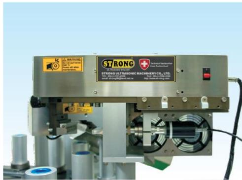
STRONG ultrasonic sealing unit is adopted on this machine. No heat radiation during sealing process, fillers are not damaged by high temperature, so Ultrasonic sealing is more suitable for biotechnical products. For better output, Switzerland-made ultrasonic units are for choice.
