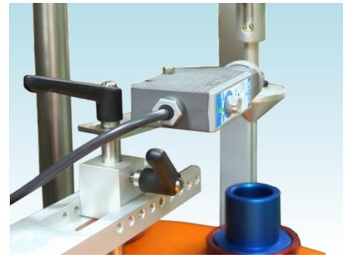
Tube Orientation is integrated into this model. Due to this new function, production speed and evenness can be improved. The Mark Sensor is adjustable for packaging different tubes. Tube rotation is driven by Step Motor beneath tubes, the surface of tubes are not wear out easily.
